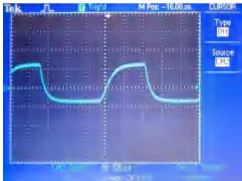
(a)  $I_{980\text{nm}}=0$ ,  $I_{1550\text{nm}}=12\text{mA}$
