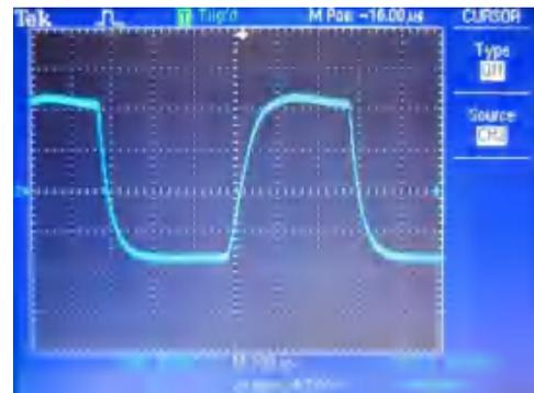
(b)  $I_{980\text{nm}}=0$ ,  $I_{1550\text{nm}}=20\text{mA}$
